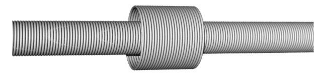
1. The shorter, larger radius coil is not connected to anything - the leads are left open. A power source drives a current in the longer, slender solenoid which changes in time according to the equation
