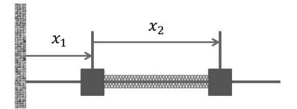
The position of  $m_1$  is measured from the wall on the left. The position of  $m_2$  is measured with respect to  $m_1$  as shown above. In terms of these coordinates, the potential energy of the spring is given by the formula
