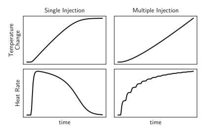
Fig. 4.1 The form of the data produced by the single injection and multiple injection methods for determination of reaction kinetics for a catalyzed reaction
