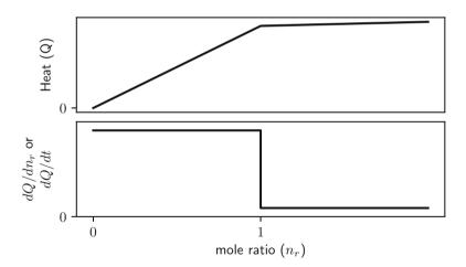
Fig. 7.4 Titration data for a quantitative 1:1 reaction
