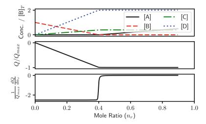
**Fig. 3.7** A reaction with coefficients on titrant and reactant both >1,  $xA + yB = zC + wD + \dots$ . Redox reactions commonly have this type of stoichiometry, e.g.,  $2MnO_4^- + 5H_2C_2O_4 + 6H^+ = 2Mn^{2+} + 10CO_2 + 8H_2O$ , although some ligand-binding reactions also have this type of stoichiometry
