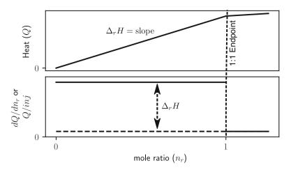
Fig. 1.2 Schematic plots of total heat to any point in the titration, Q, and of heat per increment of titrant, dQ/dn, versus the ratio of moles of titrant added to moles of titrate in the reaction vessel for a quantitative chemical reaction
