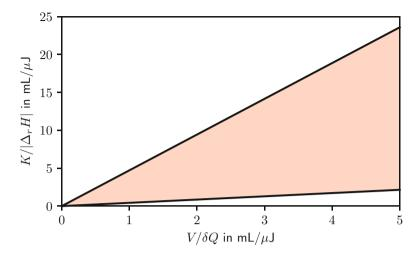
**Fig. 3.9** Upper and lower limits for the ratio  $K/|\Delta_t H|$  in simultaneous determination of the equilibrium constant and enthalpy change as a function of the reaction vessel volume and heat detection limit of the calorimeter (Hansen et al. 2011b)
