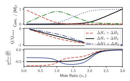
**Fig. 3.4** Species distribution and titration curves for a stepwise  $(K_1 > K_2)$  1:2 reaction, A + B = AB and  $AB + B = AB_2$ , showing the effect of the difference in  $\Delta_r H$  values on the endpoint between the two steps
