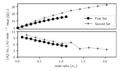
Fig. 8.1 Plot of total heat and incremental heat per mole against mole ratio for an incomplete reaction
