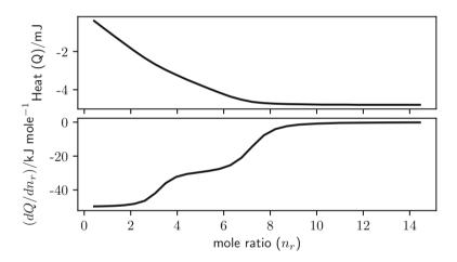
Fig. 7.2 Titration curves for titration of a small molecule into a protein with multiple binding sites
