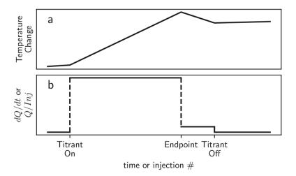
**Fig. 1.1** Schematic plots of the raw data from (**a**) temperature change and (**b**) heat conduction and power compensation calorimeters for a quantitative chemical reaction. The time constant is assumed to be zero for these plots
