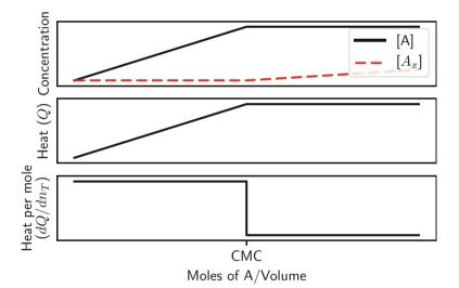
**Fig. 3.6** A self-association or aggregation reaction,  $A_x = xA$ , where *x* is an integer. Such a reaction is run with a concentrated solution of *A* as the titrant. If *x* is small, it is modeled as a cooperative reaction, i.e.,  $K_{assoc} = [A_x]/[A]^x$ , but when *x* is large, it is modeled as a phase change that occurs at a critical concentration of the aggregate, i.e., K = [A] in equilibrium with the  $A_x$  phase
