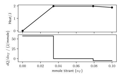
Fig. 7.1 Titration of a mixture of an amine and a sodium carboxylate with strong acid
