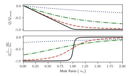
Fig. 7.5 Titration curves obtained with differing total concentrations of reactant and titrant
