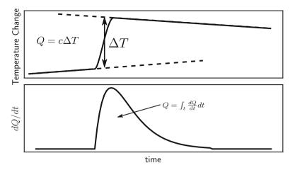
Fig. 3.8 Shows how total heat is calculated from addition of an excess of titrant to determine the amount of reactant present
