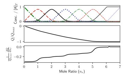
**Fig. 3.3** Species distribution and titration curves for a stepwise reaction, i.e.,  $K_1 > K_2 > K_3 > ...$ , with multiple binding sites,  $A + xB = AB_x$ , where x is an integer equal to 6, showing multiple endpoints. The total heat curve is a series of linear segments with a change in slope at the intersections
