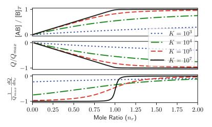
Fig. 3.2 Species distributions and plots of total heat, Q, and heat per increment of titrant, dQ/dn, for 1:1 reactions with differing equilibrium constants, K
