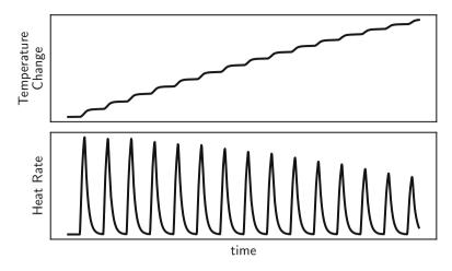
Fig. 4.2 Form of the data from titration of *A* into *B* with a slow reaction to form *AB* with a rate law, d[AB]/dt = k[A][B]
