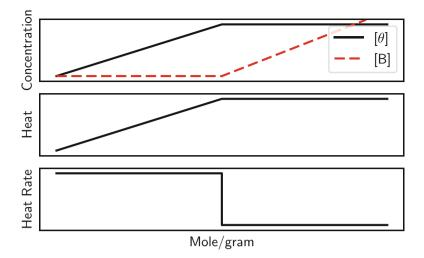
Fig. 3.5 Titration of a solution of a soluble molecule into a suspension of a solid sorbent
