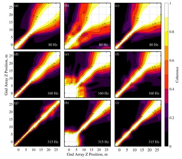
Fig. 10. Measured Coherence at the ground array for (a) 80, (d) 160, and (g) 315 Hz. The predicted coherence using the multiple-wavepacket source-model is shown for (b) 80, (e) 160, and (h) 315 Hz. In addition, the predicted coherence from the multiple-wavepacket model and uncorrelated distribution is shown for (c) 80, (f) 160, and (i) 315 Hz.
