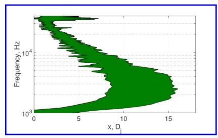
Figure 7. Apparent source region extent at the Mach 1.8 unheated jet centerline as a function of frequency as ray-traced from the probe locations within 3 dB of the maximum intensity level between z = 6.5 and 8.4  $D_{j}$ .
