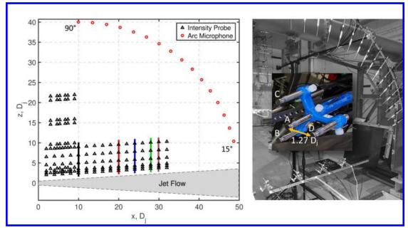
Figure 1. Left: Locations of the 40  $D_j$  polar microphone array and intensity probe measurement locations. Specific downstream distances are color-coded. Right: A four-microphone, two-dimensional intensity probe, with the microphones labeled A-D. Microphones B-D were parallel to the shear layer for most measurements. Also shown were four probes in a linear array and polar arc. The jet nozzle is located at the lower-left corner of the picture.
