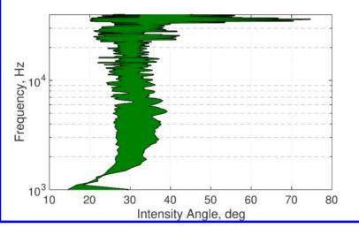
Figure 6. Measured intensity angle span within the 3-dB down region of the maximum amplitude intensity vector at the probe locations spanning z = 6.5 to 8.4  $D_j$ .
