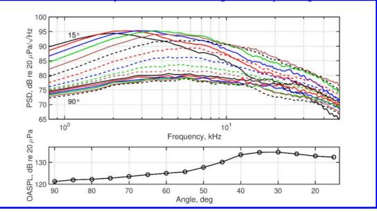
Figure 2. Power spectral densities and overall sound pressure levels at the microphone arc located at a radial distance of 40  $D_i$  and centered 10  $D_i$  downstream of the nozzle exit.
