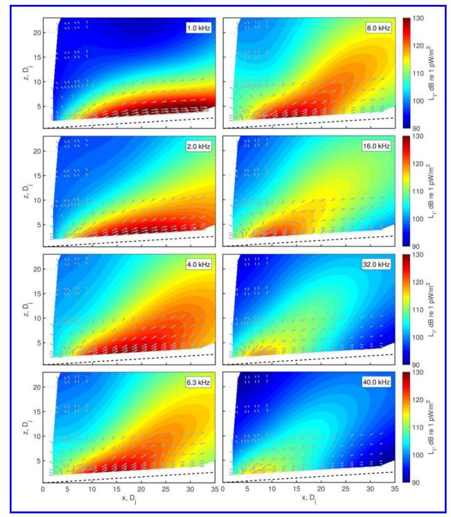
Figure 5. PAGE-calculated intensity vectors at four frequencies for a Mach 1.8, uheated jet.
