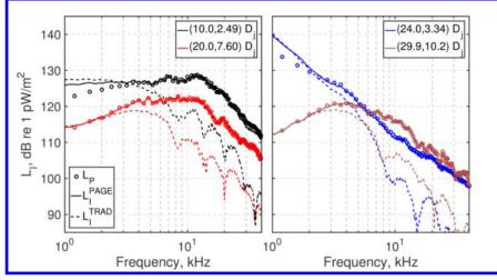
Figure 4. Intensity spectra levels, along with the sound pressure level, at the four locations shown in Fig. 4 near the Mach 1.8, unheated jet. Line colors correspond to the various downstream lines shown in Fig. 1.
