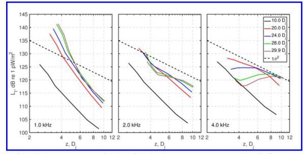
Figure 8. Radial intensity decay as a function of sideline distance, z, at the probe locations for five downstream distances; see Fig. 1.
