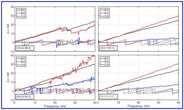
Figure 3. Unwrapped transfer function for the outer three microphone pairs using coherence-based unwrapping at locations along four downstream distances shown in Fig. 1. Irregular regions coincide with poor coherence.
