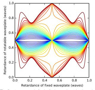
**Fig. 5.** Optimum angle for the fixed wave plate. This shows the optimum angle for the fixed wave plate in order to achieve the largest range of splitting fractions by rotating the rotatable wave plate. The contour lines are drawn every 2 deg from 2 to 44 deg. The value at the center of the plot is 0 deg, and the value at the corners is 45 deg. These values were found numerically, and used to calculate the maximum range shown in Fig. 4.
