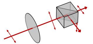
**Fig. 1.** Beamsplitting using an ideal half-wave plate and a polarizing beamsplitter. The beam entering on the left is horizontally polarized. After the polarization is rotated by the wave plate, a polarizing beamsplitter separates the horizontal and vertical components.
