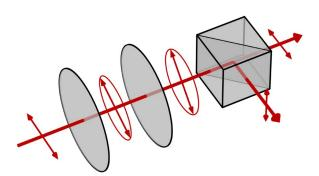
**Fig. 2.** Beamsplitting using two non-ideal wave plates. The beam entering on the left is horizontally polarized. After the polarization is modified by passing through a pair of wave plates, most generally resulting in an elliptical polarization state, a polarizing beamsplitter separates the horizontal and vertical components.
