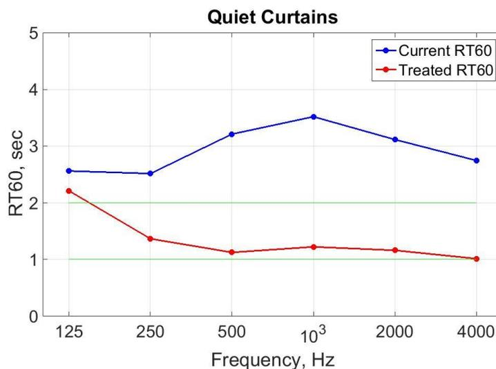
Figure 10: Effect of "Quiet Curtains" Crescent Drapes on the RT60's of the Dance Room. The red line represents the RT60 of the room after the installation curtains covering the entire north wall of the room.
