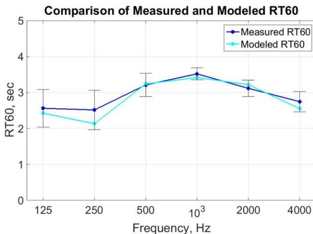
Figure 3: The modeled RT60 curve fits within the error bars of our measured data using the absorption coefficients in figure 13.
