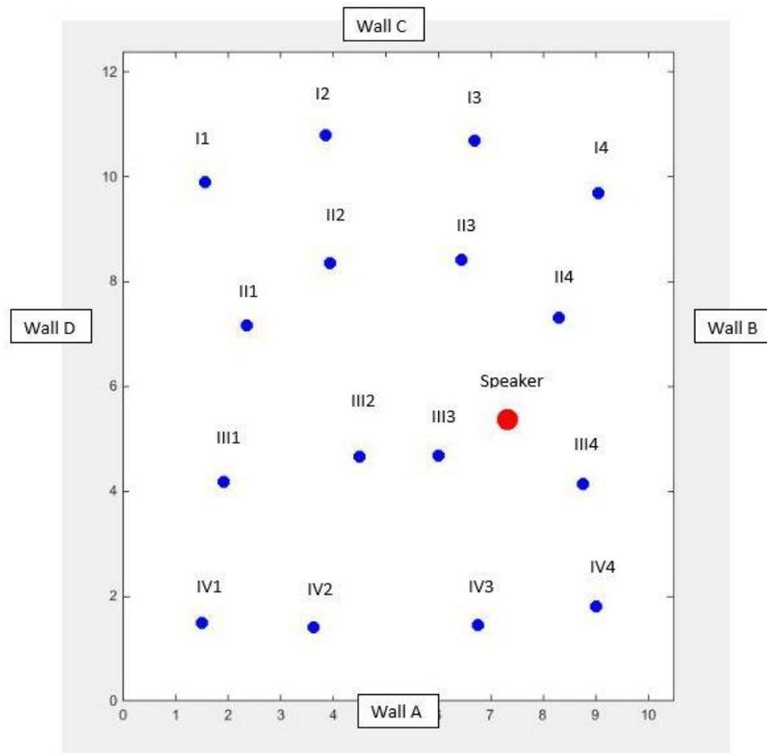
Figure 1: Locations of all microphones and speaker used in automated EASERA measurements.
