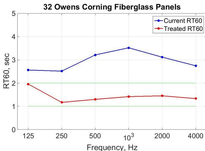
Figure 7: Effect of 32 Owens Corning Fiberglass panels on the RT60 of the Dance Room. The red line represents the RT60 of the room after the installation of the panels to the walls.
