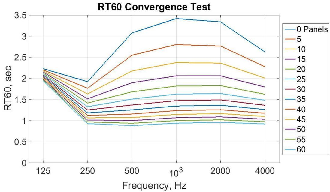
Figure 8: As fiberglass panels are added to the room, the effectiveness of each panel decreases. Each line represents 5 additional panels added to the room from 0 to 60 panels. The first 5 panels reduce the RT60 by almost 1 second, while increasing from 55 to 60
