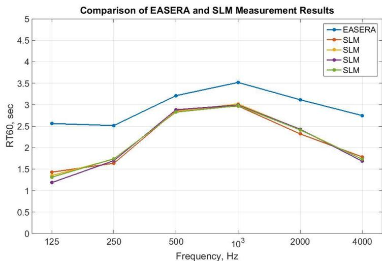
Figure 2: Plot of averaged EASERA data (blue line) and sound level meter data (other colored lines) for comparison
