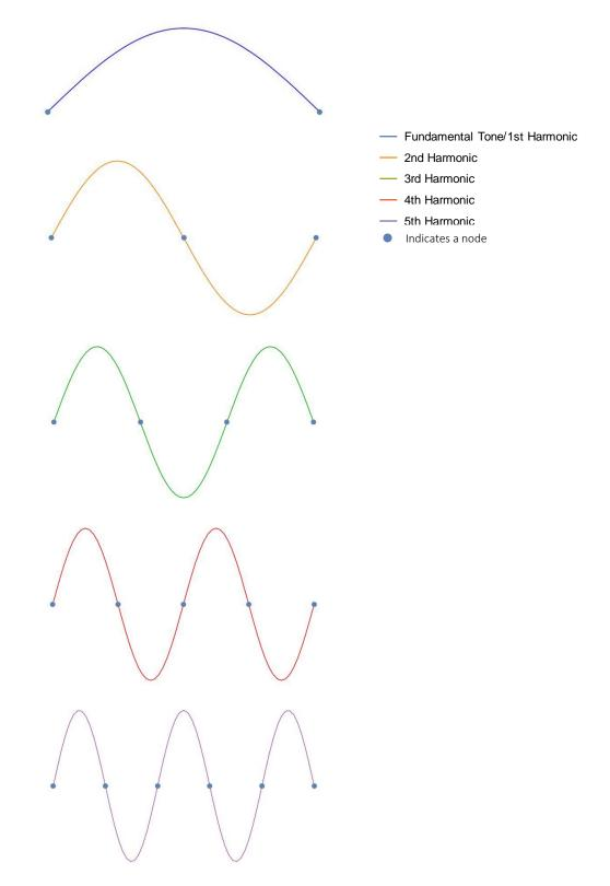
*Figure 3. The shapes of the first five harmonics of a string.*
