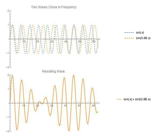
Figure 1. Two waves close in frequency interfering with each other. The interfering waves, shown as the dotted lines, result in a beat wave, shown as the solid line.
