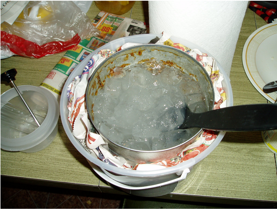
Figure 1: Tin bucket in ice cream pale, surrounded by newspaper, holding chilled solution of salt water/ice.
