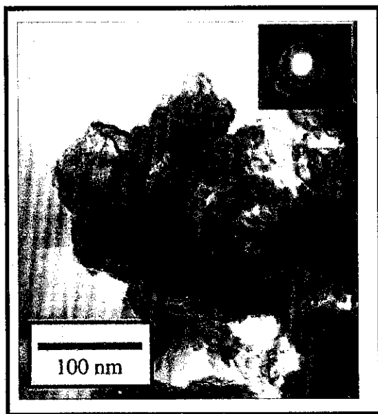
FIG. 3. A TEM image of LiH crystallites at 200 kV. The reactive gas was H_2 at \sim 0.5 mT. The inset shows the acquired diffraction pattern. The crystallites, in the imaging mode, appeared to be "moving" while under the electron beam, making their characterization difficult.
