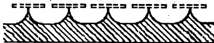
3. silicon etching continued until points formed oxide discs then removed in HF
