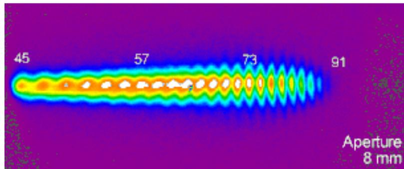
Fig. 2. (1.1 MB) Movie of harmonics generated in 120 torr helium as aperture radius varies.
