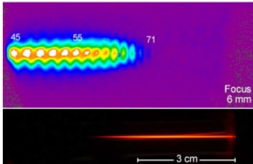
Fig. 4. (.71 MB) Movie of harmonics produced in 55 Torr of neon as focus position is varied with respect to the exit foil. The lower image is a side view of the laser focus.
