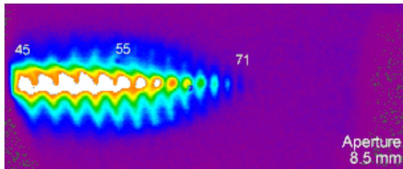
Fig.3. (1.2 MB) Movie of Harmonics generated in 55 Torr neon as aperture radius varies.
