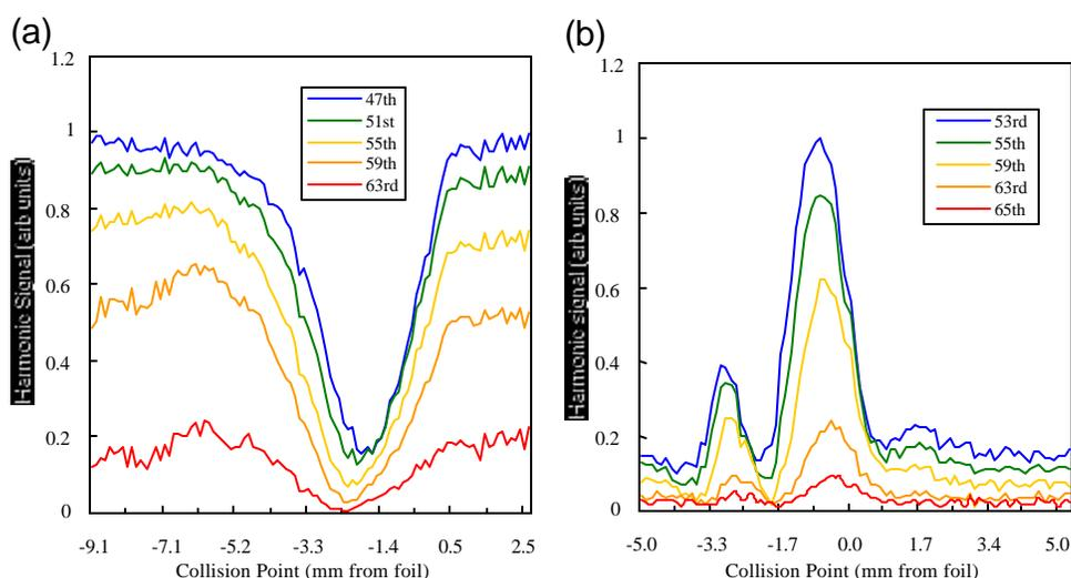
Fig. 7. Graphs of harmonic signal as a fraction of individual maximum vs. counter-propagating pulse collision point. In (b), the focus is 6mm farther upstream and pressure is 25 torr less than in (a), neon at 55 torr.
