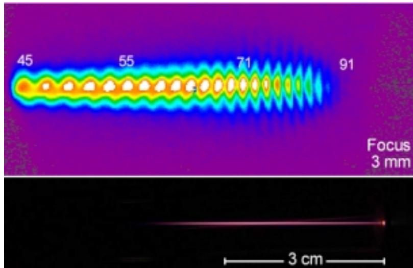
Fig. 5. (.71 MB) Movie of harmonics produced in 115 Torr of helium as focus position is varied with respect to the exit foil. The lower image is a side view of the laser focus.
