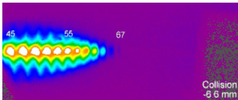
Fig. 6. (1.3 MB) Movie of harmonics in 55 torr neon as counter-propagating light sweeps through the focus.
