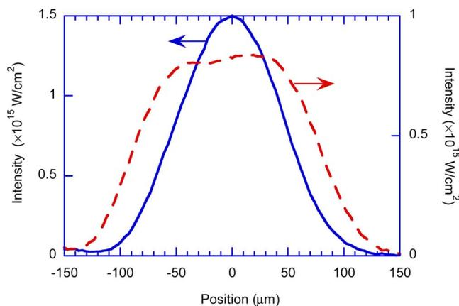
Fig. 4. (Color online) Laser intensity profile at full power captured 100 cm after the focusing mirror. The image is obtained with (dashed curve) and without (solid curve) 80 Torr helium present in the cell.
