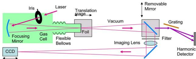
Fig. 2. (Color online) Production of high harmonics in a semi-infinite gas cell with variable exit location. Automated insertion of a mirror allows either the high harmonics or the residual laser to be observed.
