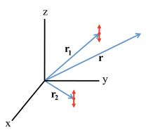
Fig. 1. Two oscillating dipoles at arbitrary locations  $\mathbf{r}_1$  and  $\mathbf{r}_2$  with orientations parallel to the *z*-axis.
