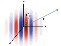
Fig. 4. (Color online) Current distribution defined by Eq. (19) at an instant in time. The direction of the current alternates with each stripe and is polarized in the *z*-direction. The internal waves propagate in the *x*-direction at speed *c* while the overall Gaussian distribution remains centered on the origin.
