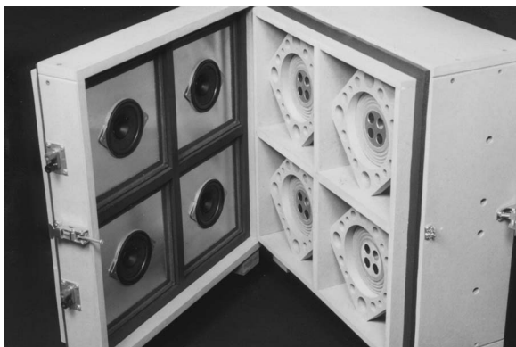
FIG. 5. A photograph of the experimental DCL array, being formed by joining the SCL actuator array to the passive transmitting diaphragm array.
