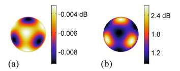
FIG. 5. (Color online) Intensity magnitude errors as a function of incidence angle for probe type "1. 3" at (a)  $ka = \pi/32$  and (b)  $ka = \pi/2$ .
