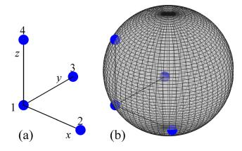
FIG. 1. (Color online) Four-microphone orthogonal probe designs with microphones freely suspended (a) and mounted on the surface of a sphere (b). Dots represent microphone locations.
