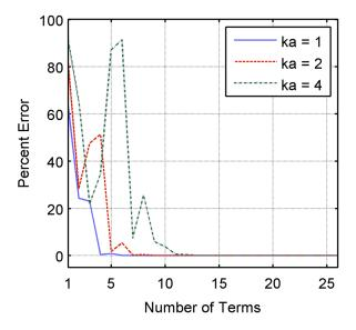
FIG. 4. (Color online) Magnitude of percent error in the scattered pressure calculation as a function of the number of terms used in the infinite expansion.
