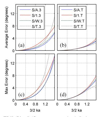
FIG. 10. (Color online) Root mean square average intensity direction errors for spherical designs using either the three points (a) or Taylor approximation (b) velocity estimate and corresponding maximum errors (c) and (d).
