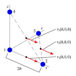
FIG. 2. (Color online) Velocity vectors needed to calculate Taylor approximation of x-direction velocity at point (h,h,h).
