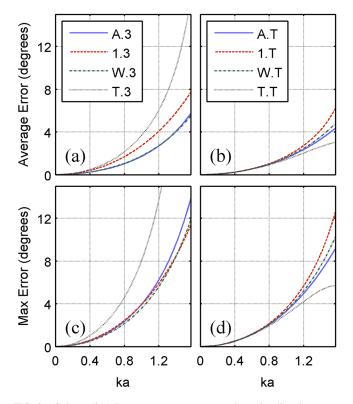
FIG. 9. (Color online) Root mean square average intensity direction errors for freely suspended designs using either the three points (a) or Taylor approximation (b) velocity estimate and corresponding maximum errors (c) and (d).
