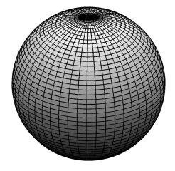
FIG. 6. Angles of incidence considered shown as the intersection points of lines of latitude and longitude.
