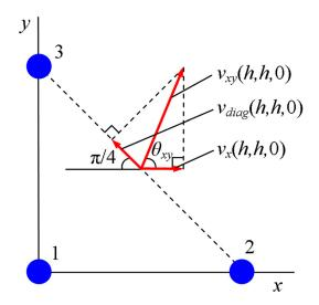
FIG. 3. (Color online) Diagram of method used to estimate *x*-direction velocity from diagonal velocity.
