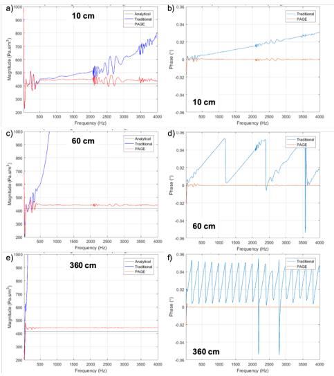
Figure 5. Impedance magnitude (left) and phase (right) using the analytical plane wave expression (black) compared to that estimated by the traditional method (blue), and the PAGE method (red) for microphone spacing, d=10, 60, and 360 cm.
