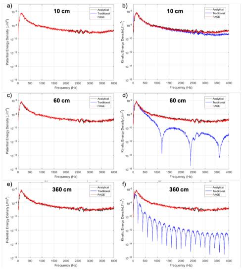
Figure 4. Potential (left) and kinetic (right) energy densities intensity using the analytical plane wave expression (black) compared to that estimated by the traditional method (blue), and the PAGE method (red) for microphone spacing, d=10, 60, and 360 cm.
