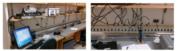
Figure 1. Photos of experimental setup. (Left) The DAQ is connected to the speaker system (on the left end of the plane wave tube), as well as the National Instruments Hardware on the shelf. The anechoic termination is visible on the far right of the image. (Right) Seven microphones spaced 10 cm apart, placed roughly in the middle of the tube. The middle microphone is not phase-matched, but the remaining six are phase-matched.
