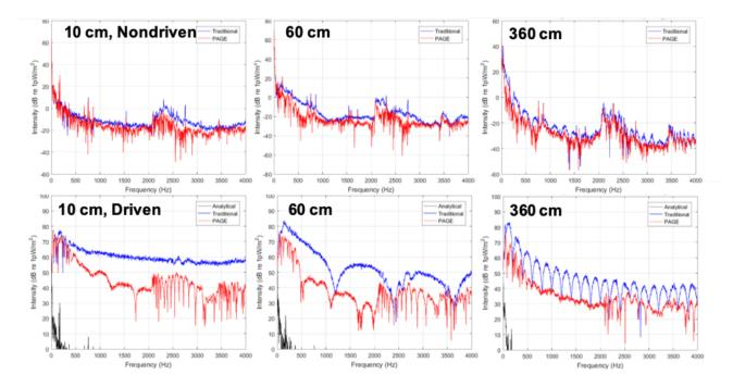
Figure 6. Reactive intensity estimated using the traditional (blue) and PAGE (red) methods for the nondriven tube (upper) and the tube driven with broadband noise (lower) for d = 10 cm (left), 60 cm (center), and 360 cm (right). (The black lines are derived from the nondriven case, not the analytical value.)
