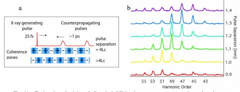
Fig. 11. Tuning the selectivity of all-optical QPM using two counterpropagating pulses, by varying their separation. The effective pulse widths of each pulse was ~300  $\mu m$ . A schematic illustrating this effect is shown in a).Enhancement occurs when the pulse separation is  $2^{N}L_{C}.$  Selectivity improves when N >1. HHG spectra from argon, in b), show the shift of the enhancement with harmonic order as the separation between the pulses is varied.
