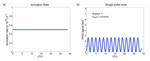
Fig. 6. Simulation of a scan of counterpropagating pulse when the strength of harmonic field and  $L_c$  do not vary along propagation. a) A constant ionization rate with propagation and b) the variation in the intensity of the detected harmonic signal for the scan of a single counterpropagating pulse, showing coherent ringing.
