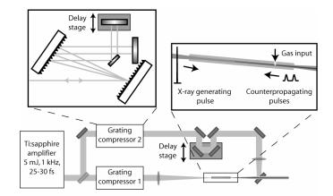
Fig. 2. Experimental setup for measuring the in-situ coherence length and implementing alloptical QPM using counterpropagating pulses.
