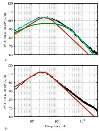
Fig. 3 PSD for 75% ETR (black) at a) 92 deg and b) 114 deg with FSS (green), LSS (red) spectra, and total modeled PSD (cyan).
