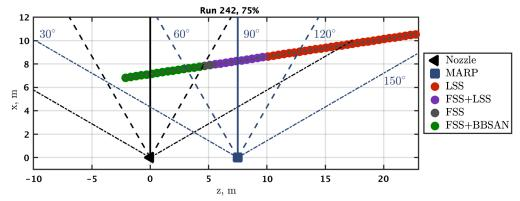
Fig. A1 Angles relative to the MARP (blue), angles relative to the nozzle exit plane (black), and the type of similarity spectra for 75% ETR at microphone locations.
