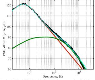
Fig. 5  $\,$  PSD for 150% ETR (black) at 152 deg compared to the LSS (red) spectrum, the FSS (green), and the total modeled PSD (cyan).
