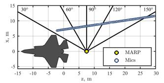
Fig. 1 Measurement geometry showing ground-based, 71 microphone array near an F-35 with inlet angles measured relative to the MARP.
