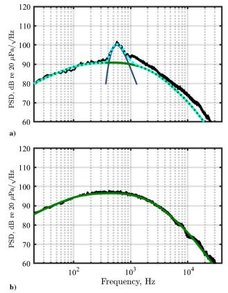
Fig. 2 PSD for 75% ETR (black) at a) 35 deg and b) 76 deg with FSS spectrum (green), Kuo et al.'s BBSAN model (blue), and total modeled PSD (cyan).
