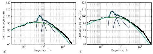
Fig. A4 F-35B PSD at a) 75% ETR (black) and b) 150% ETR decomposed into FSS spectrum (green) and BBSAN first and second harmonics (blue) with the total modeled PSD (cyan) at an inlet angle of 35.4 deg.
