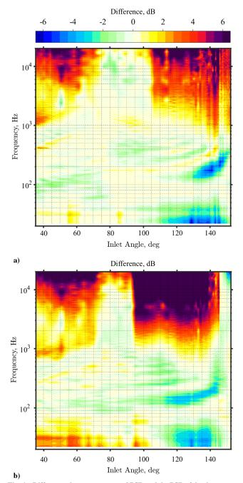
Fig. 6 Differences between measured PSD and the PSD of the three-way spectral decomposition (FSS + LSS + BBSAN) at a) 75\% ETR and b) 150% ETR.
