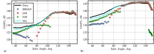
Fig. A2 F-35B OASPL (black) at a) 75% ETR and b) 150% ETR with the modeled spectral components: LSS (red), FSS (green), BBSAN (blue), and combination (cyan).
