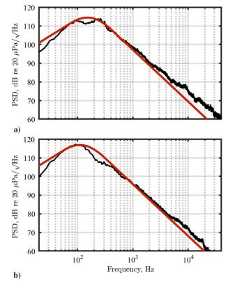
Fig. 4 PSD for 75% ETR (black) at a) 133 deg and b) 146 deg compared to the LSS (red) spectrum.
