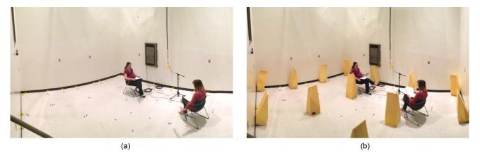
FIG. 1. (Color online) Interviewer (left) and subject (right) in the reverberation chamber with (a) 0 and (b) 16 acoustically absorptive wedges present.
