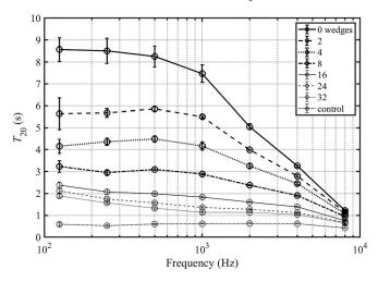
FIG. 2. Spatially averaged  $T_{20}$  values for all unoccupied experimental conditions, reported in octave bands.
