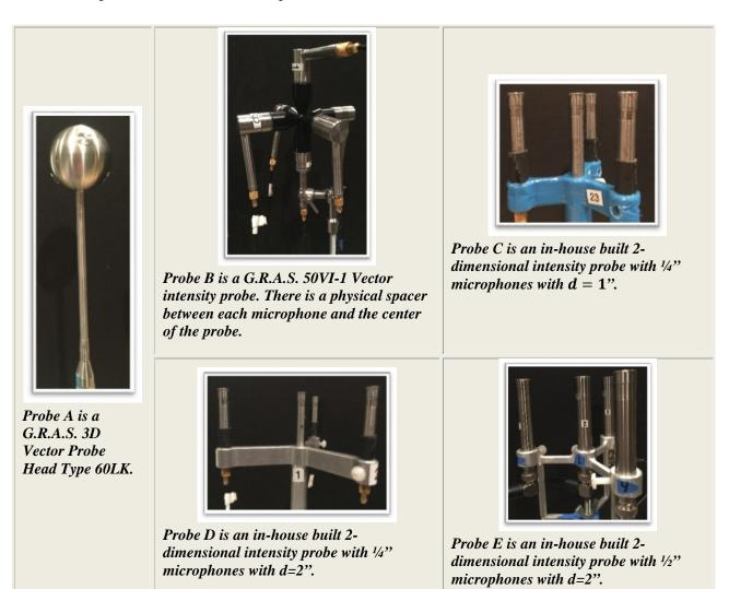
Figure 1: This figure contains a photo of each of the five intensity probes. Along with the photo is the probe's designation and description.
