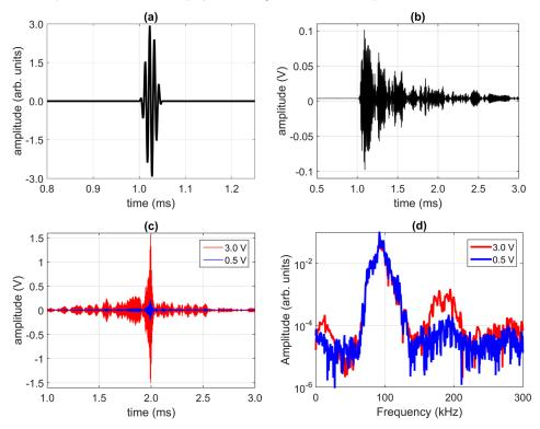
Fig. 2. (Color online) Typical time domain signals of a TR experiment used in this study: (a) 3.0 V, 100 kHz pulse signal broadcast from one source to the laser position; (b) typical received signal by the laser during the forward step; (c) typical TR focal signals obtained by the laser for 0.5 and 3.0 V inputs; (d) typical spectra of the focal signals obtained at a damaged location.
