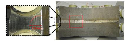
Fig. 1. (Color online) Photograph of the sample under test (on the right). Solid red line colored box indicates the approximate scan area. The dashed line black box (on the left) shows an edge view photograph of the side of the sample with a red dashed line indicating the extent of a barely visible crack.
