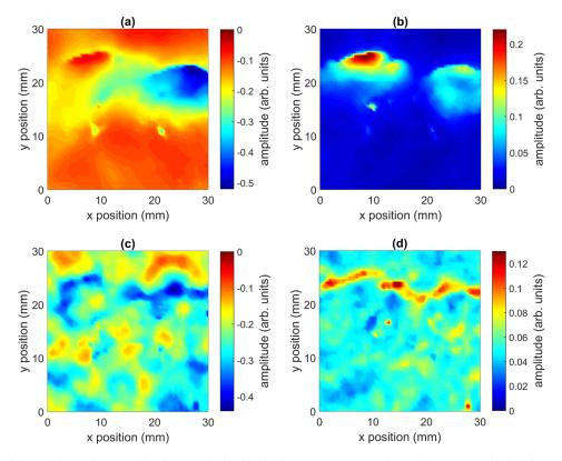
Fig. 3. (Color online) SSM focal maps obtained using the TREND. (a) 100 kHz pulse source excitation, image spans the fundamental band of 70–130 kHz. (b) 100 kHz pulse source excitation, image spans second harmonic band of 170–230 kHz. (c) 200 kHz pulse source excitation, image spans the fundamental band of 150–250 kHz. (d) 200 kHz pulse source excitation, image spans the second harmonic band of 350–450 kHz.
