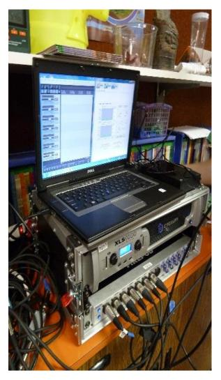
Figure 5. Microphones connected to the digital audio workstation.
