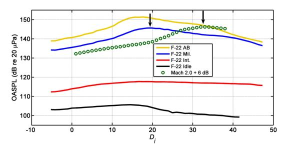
Fig. 2 – Unweighted OASPLs for all engine conditions of the F-22, recorded along the groundbased microphone array, as a function of distance downstream in nozzle diameters  $D_j$ . The circles indicate the unheated, Mach 2.0 laboratory data (described in Section 3) adjusted by 6 dB to account for the absence of ground reflections in the anechoic chamber. The arrows indicate the maximum OASPLs for the laboratory jet and the F-22Aat military power.
