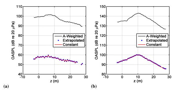
*Fig.* 5 – *Hearing protection gains applied to the A-weighted data for (a) idle and (b) military engine conditions.*
