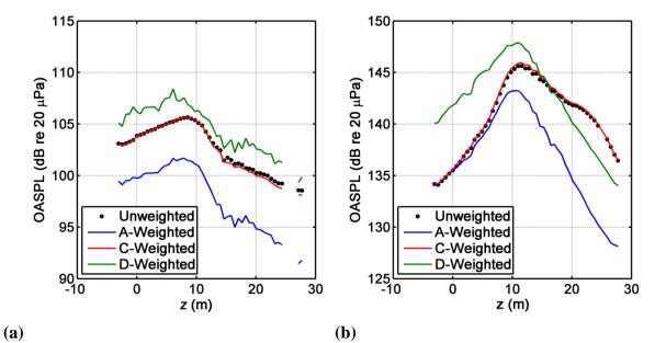
Fig. 4 – Weighted OASPLs for (a) idle and (b) military engine conditions.
