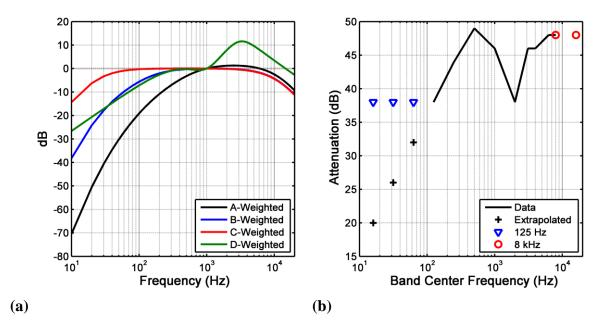
*Fig. 3 – (a) Weighting curves and (b) octave-band attenuation for 100% inserted foam plugs with muffs worn by properly trained personnel. The markers represent different ways of handling the data outside the 125 Hz – 8 kHz bandwidth.*
