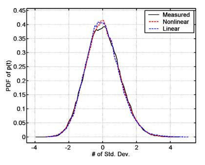
Figure 2: Probability density function of 304.8-m AB waveforms.
