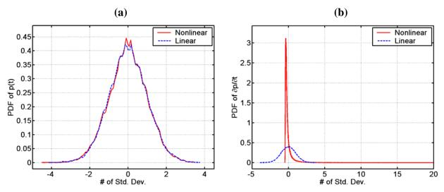
**Figure 6:** Probability density functions of the (a) waveforms and (b) waveform time derivatives at 500 m. Positive derivative values for the nonlinearly-propagated waveform continue out to nearly 79 standard deviations.
