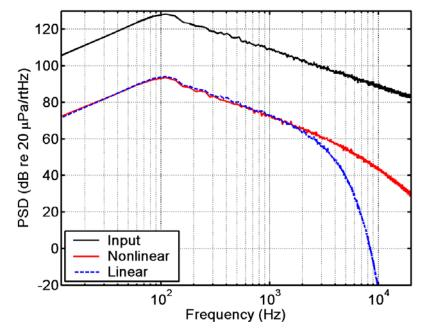
**Figure 4:** Power spectral density (PSD) of the input shaped random noise at 10 m and the linearly- and nonlinearly-predicted spectral densities at 500 m. The linear prediction exceeds -200 dB re  $20 \,\mu$ Pa/ $\sqrt{Hz}$  at 20 kHz.
