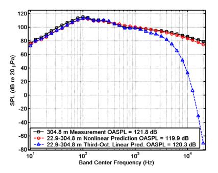
Figure 1: Measured and predicted third-octave spectra at 304.8 m and one engine at afterburner.
