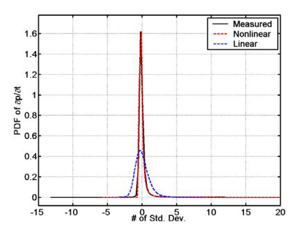
**Figure 3:** Probability density functions of the 304.8-m AB waveform time derivatives. The positive tails for both the measured and nonlinearly-predicted distributions extend out to approximately 63 standard deviations.
