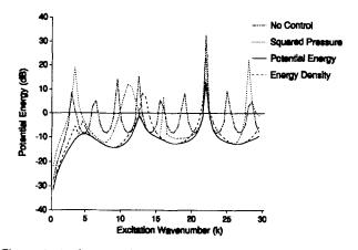
Figure 4. Total potential energy using multiple sensors. Squared pressure sensor locations: x = 0.02, 0.2, 0.4, 0.6, 0.8, 0.98L. Energy density sensor location: x = 0.5L.
