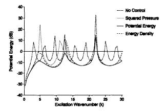
Figure 3. Total potential energy in the duct. For the squared pressure and energy density, the discrete sensor is located at the position x = 0.872L.
