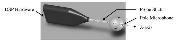
Figure 1: Energy Density Probe
