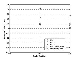
Figure 14: Calibration Error at 500 Hz and 114 dB
