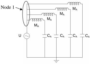
Figure 3: Equivalent Circuit Model
