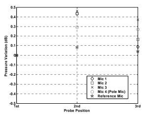
Figure 16: Calibration Error at 2000 Hz and 110 dB
