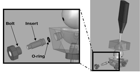
Figure 10: CAD Model of Attachment
