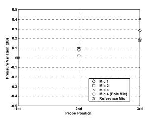
Figure 15: Calibration Error at 1000 Hz and 114 dB
