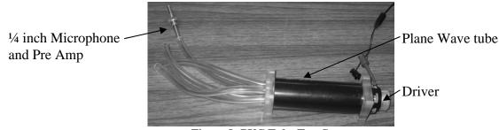
Figure 8: PVC Tube Test Setup
