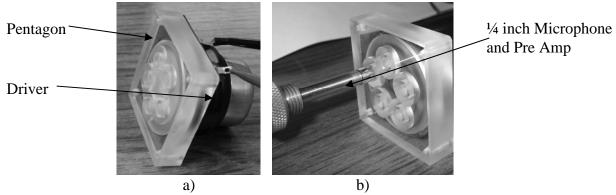
Figure 5: a) Microphone Measuring Pressure at Pentagon port b) Pentagon Attached to Driver
