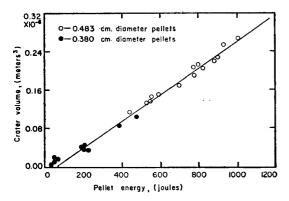
FIG. 3. Relationship between crater volume and pellet energy when mild steel (1040) spheres are fired into semi-infinite targets of the same composition.
