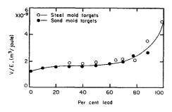
FIG. 10. Crater volume per unit energy, V/E, for different alloys plotted against composition.
