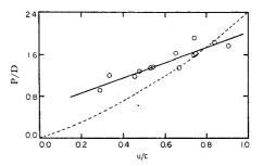
FIG. 6. Penetration in units of the pellet diameter plotted against u/c (Mach number) for tin spheres and targets.
