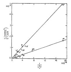
FIG. 5. Volume per unit energy plotted against the parameter,  $1/c^2\rho$ , for several pure metals.
