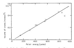
FIG. 2. Relationship between crater volume and pellet energy when zinc spheres are fired into semi-infinite zinc targets.
