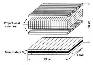
FIG. 1. Schematic view of hodoscope and scintilla-tors.
