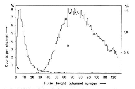
FIG. 2. Measured pulse height distributions for (a) particles of unit charge and (b) quarks. The distribution for quarks was simulated by observing particles of unit charge in counters built to  $\frac{1}{9}$  scale.
