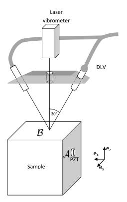
FIG. 2. Experimental setup. The DLV used to obtain the in-plane components is mounted on a rotational stage in order to measure the x and y components individually. The DLV and normal LV are focused coincidently and synced to obtain in-plane and out-of-plane components simultaneously. For the experiments reported here  $x_A = x_B$ , the unit vectors for which are shown.
