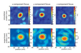
FIG. 5. (Color) Three component focusing with  $R_x^{(1)}(-t) + R_y^{(1)}(-t) + R_x^{(1)}(-t)$ . Model (top row) and experimental (bottom row) results. Magnitude of the three velocity components of motion  $R_x^{(2)}(t) = v_x$ ,  $R_y^{(2)}(t) = v_y$ , and  $R_z^{(2)}(t) = v_z$ . The color scales are normalized to the maximum amplitude in each respective component. Note the near identical focal structure for each component.
