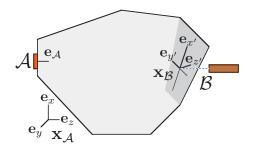
FIG. 1. (Color) Pictoral representation showing a sample with a source transducer capable of emitting a signal unidirectional in the direction  $e_A = e_z$  in the frame  $x_A$  at A; and a laser vibrometer receiver measuring the components in the  $x_B$  frame at B.
