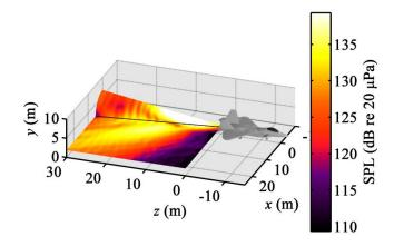
Figure 3: MSTR SONAH reconstruction in the vicinity of the jet for military power, 125 Hz. Levels are shown on a half conical surface (toward the side of the measurement) at the approximate location of the shear layer edge and over a plane at y = 1.9 m, the height of the centerline of the jet.
