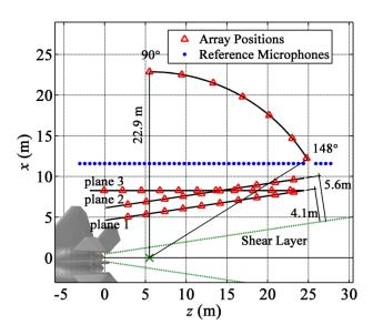
**Figure 1:** Schematic of the measurement locations, relative to the aircraft. The estimated shear layer boundary is marked by green dashed lines, and the green "x" delineates the estimated maximum noise source region and the center of the arc.
