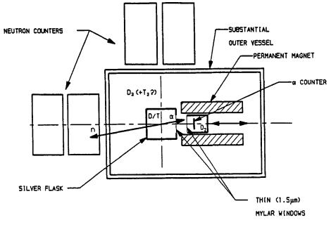
Fig. 1. Apparatus for measuring W<sub>s</sub>.
