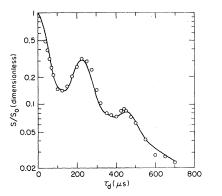
FIG. 5. Spin-echo amplitude  $S/S_0$  at  $H_0/v_0=1.138$  kG/MHz,  $v_0=74$  MHz, and T=4.2 K. Solid line is the best fit to Eq. (10). See Table I.
