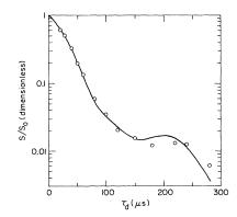
FIG. 7. Spin-echo amplitude  $S/S_0$  at  $H_0/v_0=1.138$  kG/MHz,  $v_0=74$  MHz, and T=77 K. Solid line is the best fit to Eq. (10). See Table I.
