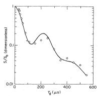
FIG. 9. Spin-echo amplitude  $S/S_0$  at  $H_0/v_0=1.138$ kG/MHz,  $v_0=8.4$  MHz, and T=4.2 K. Solid line is the best fit to Eq. (10). See Table I.
