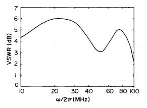
FIG. 3. The VSWR of the broadband NMR probe.
