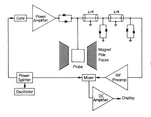
FIG. 1. Block diagram of pulse spectrometer.
