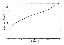
FIG. 3. Surface conductance of a copper wire in petroleum ether as a function of applied hydrostatic pressure. The pressure is hydrostatic below 30 kbars.
