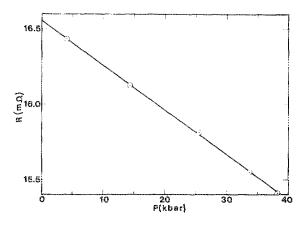
FIG. 2. Resistance of a copper wire vs pressure extrapolated to zero measuring current.
