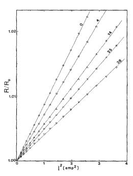
FIG. 1. Resistance of a copper wire vs the square of the measuring current for the wire in petroleum ether at various pressures in kbars indicated on each curve.
