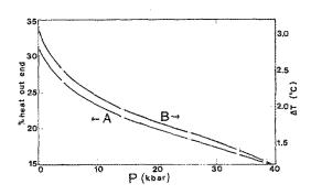
FIG. 4. (A) The percentage of the joule heat that leaves the wire through each end. (B) The temperature discontinuity between the wire and surrounding fluid at the center of the wire with 1 A flowing.
