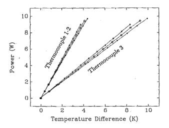
FIG. 2. The power vs temperature difference corresponding to several different pressures in kbar (dot—5, circle—10, asterisk—38) for natural pyrophyllite.
