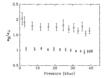
FIG. 4.  $\kappa_{\parallel}/\kappa_{\perp}$  vs pressure for natural (circles) and baked (squares) pyrophyllite.
