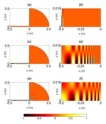
FIG. 4. (Color online) Wave propagation images (spatial distribution of pressure at an instant in time) for a single-cycle 16 kHz excitation signal in the (0,1) mode. Wave propagation for the full spatial model is shown to scale in (a), (c), and (e). Wave propagation solely within the pipe is shown in (b), (d), and (f). The times for each subplot are as follows: (a) and (b) 0.0625 ms, (c) and (d) 1.5 ms, (e) and (f) 2.2 ms.
