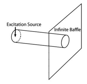
FIG. 1. Illustration of the physical domain used to study transient radiation from a finite-length pipe.
