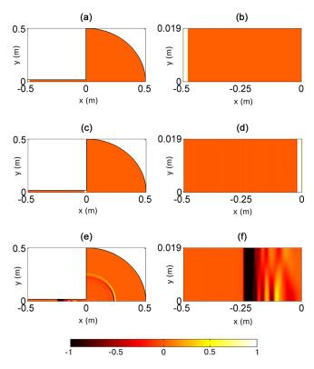
FIG. 3. (Color online) Wave propagation images (spatial distribution of pressure at an instant in time) for a single-cycle 16 kHz excitation signal in the (0,0) mode. Wave propagation for the full spatial model is shown to scale in (a), (c), and (e). Wave propagation solely within the pipe is shown in (b), (d), and (f). The times for each subplot are as follows: (a) and (b) 0.0625 ms, (c) and (d) 1.5 ms, (e) and (f) 2.2 ms.
