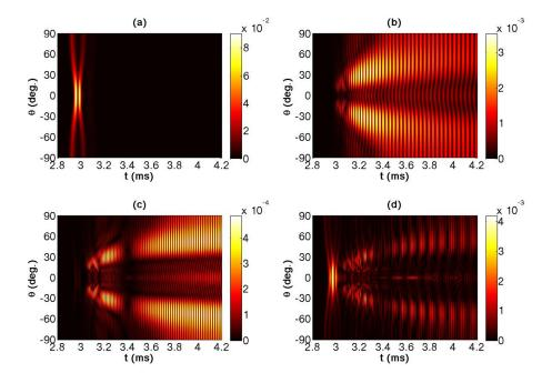
FIG. 5. (Color online) Far-field radiation (pressure magnitude) measured at 0.508 m from the exit of the pipe as a function of angle and time for various modes of the 16 kHz gated sine wave. (a) (0,0) mode. (b) (0,1) mode. (c) (0,2) mode. (d) Combination of several modes, where the spatial component of the normal acceleration is given as  $\cos(3\pi r/a)$ .
