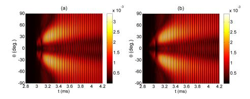
FIG. 6. (Color online) Far-field radiation (pressure magnitude) measured at 0.508 m from the exit of the pipe as a function of angle and time for the (0,1) mode of the 16 kHz gated sine wave. (a) Finite difference simulation result [same as Fig. 5(b)]. (b) COMSOL simulation result.
