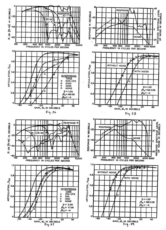
FIG. 36. System I with interfering tone at 78.2 db above threshold, for three different tone frequencies. FIG. 37. System I with interfering tone at 60.8 db above threshold, for three different tone frequencies.
