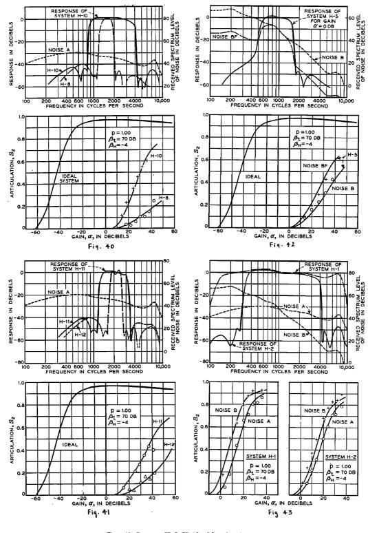
FIG. 40. Systems H-8, H-10 with noise A. FIG. 41. Systems H-11, H-12 with noise A. FIG. 42. System H-5 with noises B and BF. FIG. 43. Systems H-1, H-2, with noises A and B.
