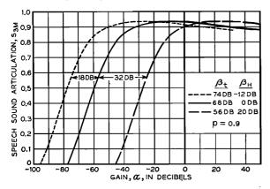
FIG. 47. Calculated articulation vs. gain for commercial system in quiet with range of talking level  $\beta_t$  and hearing loss  $\beta_H$ .
