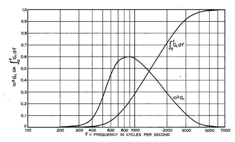
FIG. 9. The functions  $G_1$ and  $\int_0^J G_1 df$ .  $G_1$  is the frequency weighting factor for loudness, when speech is at the threshold of audibility. (See also Fig. 50 and Table VIII.)
