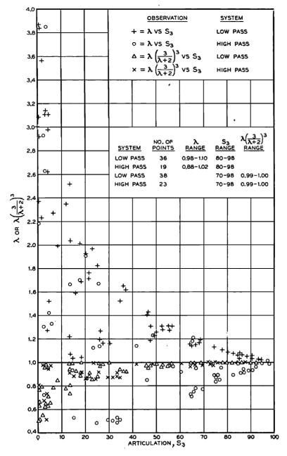
FIG. 2. Observed values of  $\lambda$  and  $\lambda(3/\lambda+2)^3$  vs. syllable articulation  $S_8$  for filter systems.
