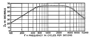
FIG. 11. Level  $Z_F$  of each critical band of undistorted speech in decibels above threshold, when the speech is at the optimum level for interpretation.
