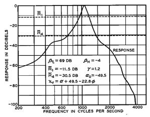
FIG. 10. Response of resonant system II-RN-1060, with weighted averages  $\vec{R}_1$  and  $\vec{R}_4$  and values of  $\gamma$ ,  $\alpha_0$  and  $x_{T}$ .
