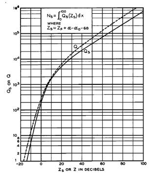
FIG. 53. The functions  $Q_s$  vs.  $Z_s$  and Q vs. Z.
