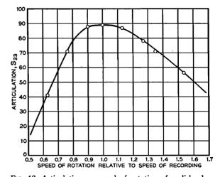
FIG. 18. Articulation vs. speed of rotation of a disk phonograph record of speech: Observations (points) and calculations (curve).
