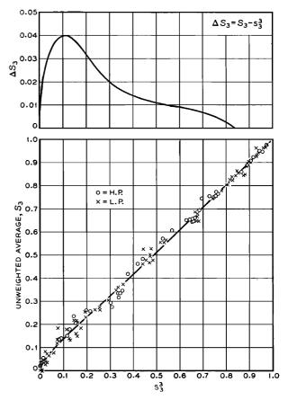
FIG. 3. Unweighted average syllable articulation  $S_3$  and  $\Delta S_3$  vs. cube of speech sound articulation  $s_3^3$  for filter systems.
