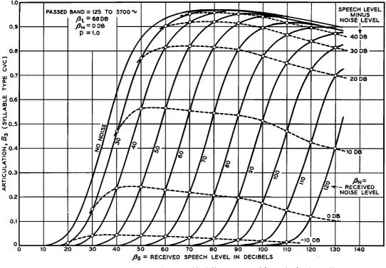
FIG. 49. Calculated articulation vs. gain for an ideal filter system with a noise having uniform spectrum level at all passed frequencies.
