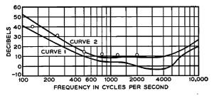
FIG. 8. Minimum audible pressure levels for typical listener of the articulation test crews, in decibels from 0.0002 dyne/cm<sup>2</sup>. Curve 1=Monaural minimum audible field. Curve 2=Monaural minimum audible pressure level under earphone. Points=Observations for 1919-1920 crew.
