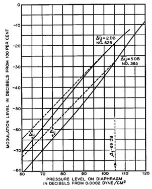
FIG. 20. Output vs. input characteristics of No. 395 and No. 625 carbon type microphones tested in a constant sound field at frequency 1000 c.p.s.
