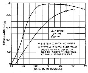
FIG. 17. Articulation of 1919-1920 high quality system without and with loud interference by a pure tone at frequency 2000 c.p.s.: The curves have been drawn to represent the points (observations).
