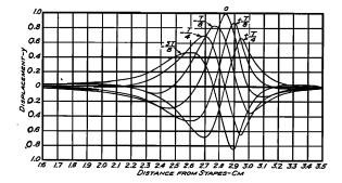
FIG. 8. Shape of basilar membrane during vibration at times which are successively  $\frac{1}{8}$  of a period apart.
