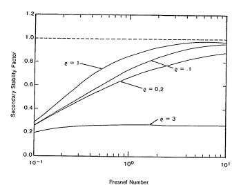
Fig. 7. Plots of the stability factor  $F_w$  of the secondary beam parameter vs Fresnel number for the selected values of  $\rho$ .
