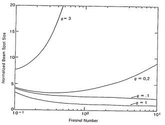
Fig. 2. Plots of the normalized beam spot size  $kW_s^2/2L$  vs Fresnel number N for various values of  $\rho = L/R_m$ .
