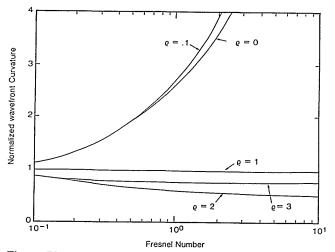
Fig. 3. Plots of the normalized wave-front curvature  $R_s/L$  vs N.
