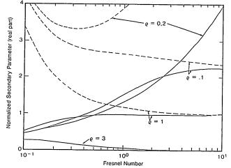
Fig. 4. Plots of the real part of the normalized secondary beam parameter  $kw_s^2/2L$  vs N. For resonators that have confined beam modes at large N, these curves approach each other as N increases.
