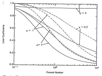
Fig. 8. Plots of the loss coefficients  $\wedge_{0,0}$  (solid curves) and  $\wedge_{0,1}$  (dashed curves) for the selected values of  $\rho$ .
