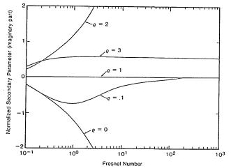
Fig. 5. Plots of the imaginary part of the normalized beam parameter vs N. For resonators with confined beam modes at large N, these curves approach zero as N increases.
