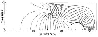
FIG. 6. A computer-drawn graph of the poloidal magnetic field lines in the neighborhood of a compressed high beta plasma. The positions of the I and C coils and plasma surface are shown for an equilibrium configuration of the plasma.
