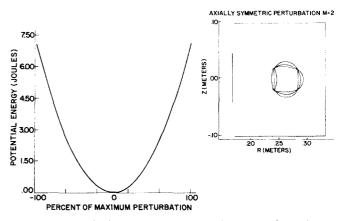
FIG. 8. A graph showing the work done by the net force (excluding the perturbing force) acting on the plasma surface during an axially symmetric perturbation. The work is interpreted as a potential energy and is plotted to show the minimum at equilibrium. The M=2 perturbation is shown together with its potential well: The abscissa shows percent of the maximum perturbation.
