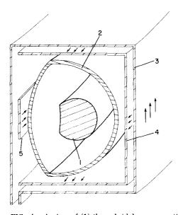
FIG. 4. A view of (1) the poloidal cross section of a plasma with two limit cycles. Also shown are (2) the vacuum envelope, (3) the  $\theta$  coil, (4) the C coil, and (5) the I coil. The directions of the currents in the coils are indicated with arrows.
