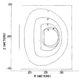
FIG. 5. The plasma surface position in the poloidal plane of a topolotron compression. Positions shown are for (1) 0.01, (2) 0.32, (3) 0.76, (4) 1.05  $\mu$ sec after the compression was initiated, and (5) the equilibrium position of the plasma. Contour (2) is near the end of the snowplow phase and contour (4) is near the crowbar time.
