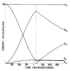
FIG. 7. A graph showing the energy in  $(E_c)$  the capacitors,  $(E_m)$  the magnetic field,  $(E_p)$  the plasma,  $(E_R)$  dissipated in the resistance and  $(E_T)$  the total energy, as a function of time during the simulated plasma compression. Note the change in the time scale after crowbarring indicated by the dotted line.
