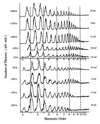
FIG. 2. Harmonic spectra generated in 5 Torr of argon for fixed peak laser intensity of  $5 \times 10^{14} \text{ W/cm}^2$  and for various laser pulse chirps.
