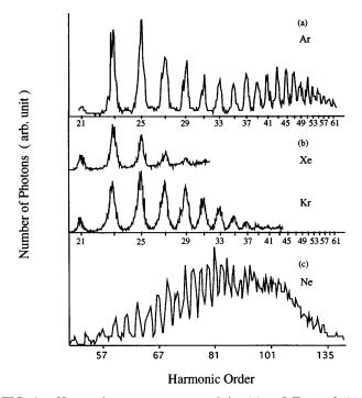
FIG. 1. Harmonic spectra generated in (a) ~5 Torr of Ar, and (b) 2 Torr of Kr and Xe, with peak laser intensity  $5 \times 10^{14}$  W/cm<sup>2</sup>. (c) Harmonic spectra generated in ~10 Torr of Ne with peak laser intensity  $2 \times 10^{15}$  W/cm<sup>2</sup>. The relative intensities of (a)–(c) should not be compared directly.
