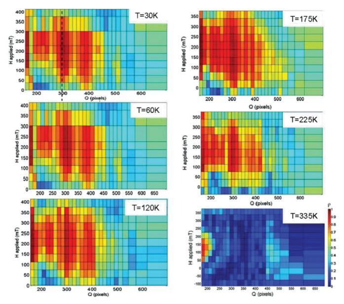
FIG. 4. (Color online) Correlation maps at different temperatures 30, 60, 120, 175, 225, and 335 K. All maps are measured along the ascending branch of the magnetization loop.
