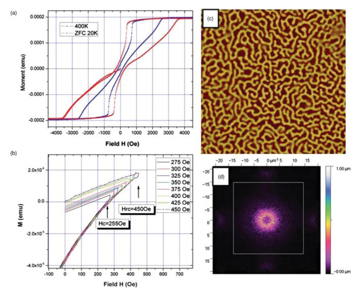
FIG. 1. (Color online) (a) Magnetization loop measured by VSM, at 400 K ( $T > T_B$ ) and in ZFC state at 20 K after demagnetization at 400 K; (b) measurement of the remanant coercive  $H_{RC}$  point by gradual field increment; (c)  $10 \times 10 \ \mu\text{m}^2$  MFM image measured at room temperature in the remanant state, showing the typical magnetic domain pattern which will later be imprinted; (d) Fourier transform of the MFM image shown in (c).
