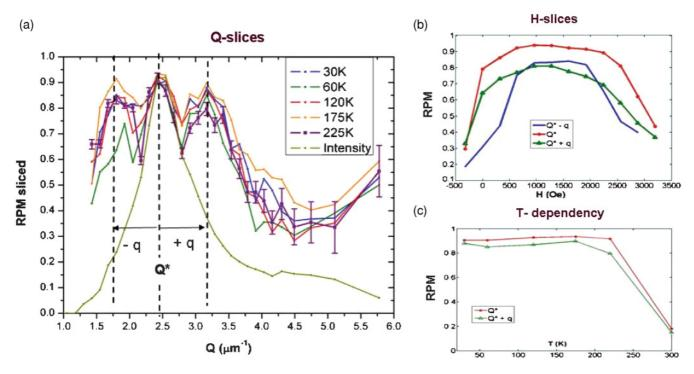
FIG. 5. (Color online) Q and H slices through maps and temperature dependency. (a) Q slices from the  $\rho(Q,H)$  maps, in the coercive region  $(H \sim H^*)$ , at different temperatures from 30 up to 225 K, and slice from the intensity I(Q,H) at 225 K for comparison. Error bars are indicated on the 225 K slice. (b) H slices from the  $\rho(Q,H)$  map at 225 K, at  $Q=Q^*$  and  $Q=Q^*\pm q$ . (c) Maximum correlation value  $\rho$  with temperature T, for  $Q=Q^*$  and  $Q=Q^*+q$ .
