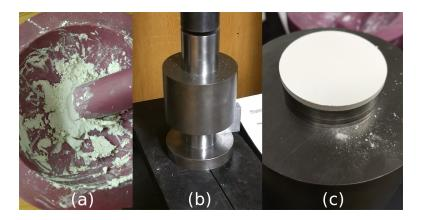
**Figure 2.1** Target preparation process including (a) powder during mixing, (b) placement in hydraulic press, and (c) fully formed target ready for firing. Note the rectangular aluminum spacer used in (b) to keep the outer section of the die from falling down.
