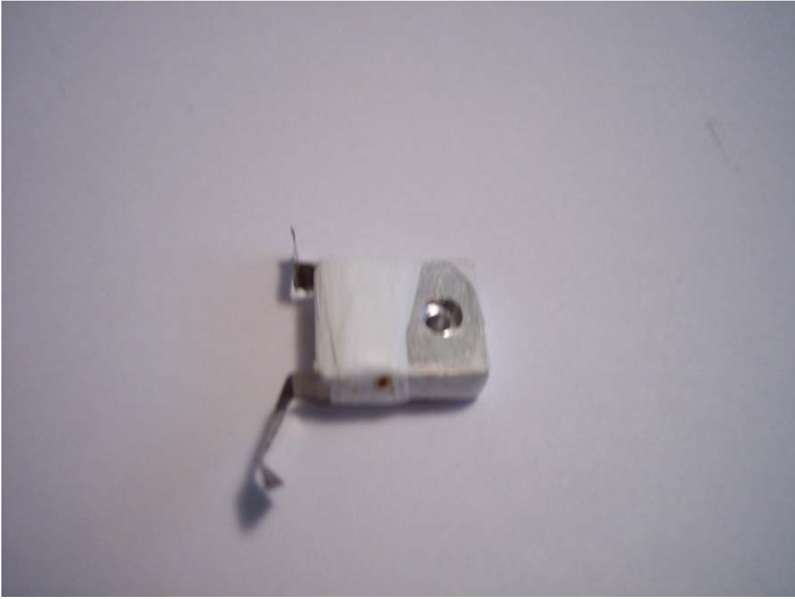
Figure 7: Aluminum block with zirconium and Teflon sealant
