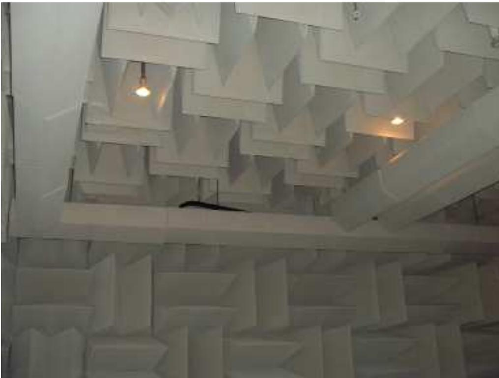
**Figure 2.3** Photograph of the acoustical absorptive wedges installed on the gantry.
