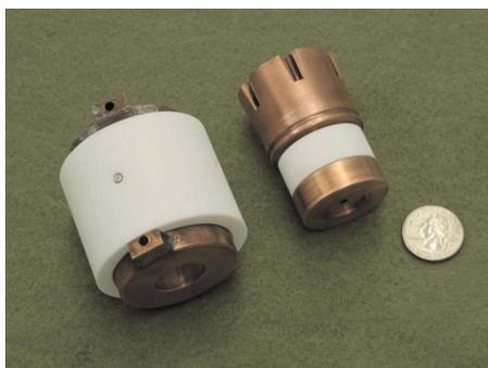
FIG. 2. (Color online) The assembled mounting rings (left) and ion source (right).
