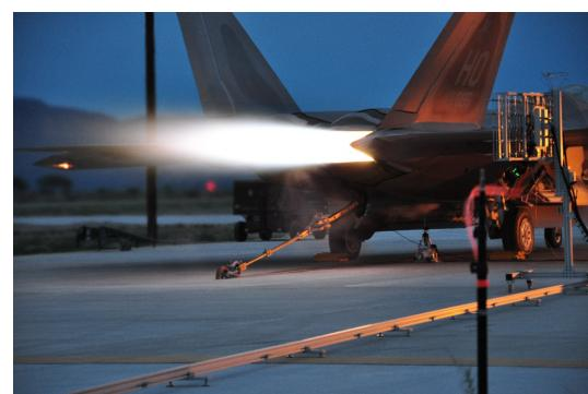
*Fig. 1—Measurement setup, with F-22 tethered to concrete run-up pad. The rectangular microphone rig is visible on the right, atop an aluminum guide rail.*
