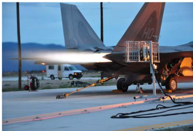
Figure 2 BRRC 90-microphone array, scanning the near field of the jet on an F-22 Raptor.
