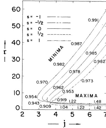
FIG. 1. As a function of the angular momentum constant  $j$  [cf. Eq. (6b)], the radial position coordinate,  $r = r/M$ , of the effective potential maxima and minima for a spinning test particle executing equatorial motion in a Schwarzschild field. The curves for negative values of  $j$  are obtained by letting  $j \rightarrow -j$  and  $s \rightarrow -s$ .
