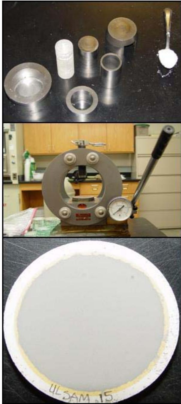
**Fig. 5. Top:** shows the set of dies, and a spoonful of the cellulose. **Middle:** the hydraulic press used to compress the sample using a seven ton force. **Bottom:** the final pressed pellet ready for WDXRF.
