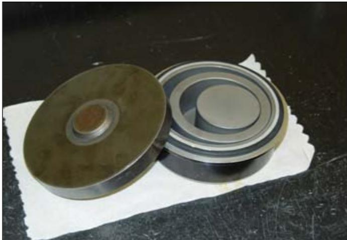
**Fig. 8.** The tungsten vessel used for pulverizing the majority of the samples for production of pressed pellets.
