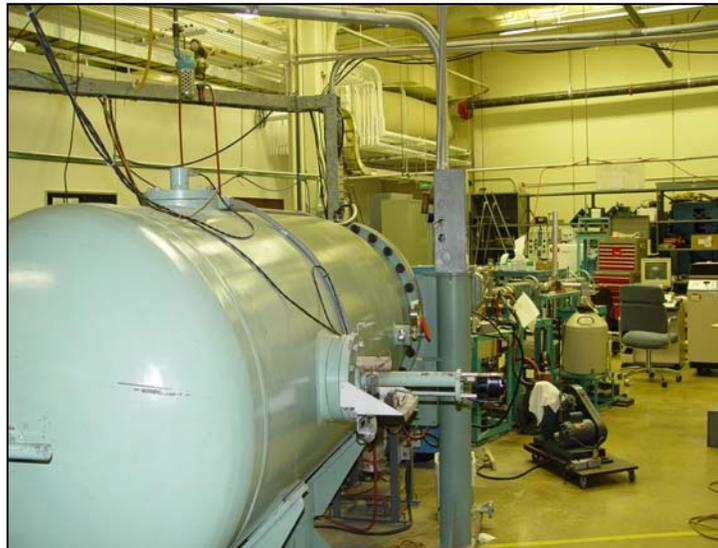
**Fig. 1.** The Van De Graff accelerator used for PIXE spectrometry, The Si(Li) detector can also be seen towards the back.
