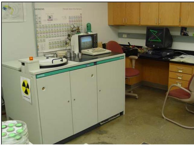
**Fig. 6.** A picture of the Siemens SRS 303 Wavelength-dispersive XRF, and the analysis computer.
